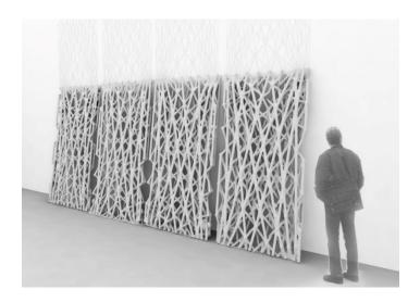
Each "tapestry" is reinforced with a braided carbon fiber armature that leverages techniques from traditional lacemaking—those that usually produce pictorial motifs—into purposeful forms that adopt a material and structural function. The project builds on previous research employing a hybridized computational and analogue workflow for the design and fabrication of each underlying armature.
